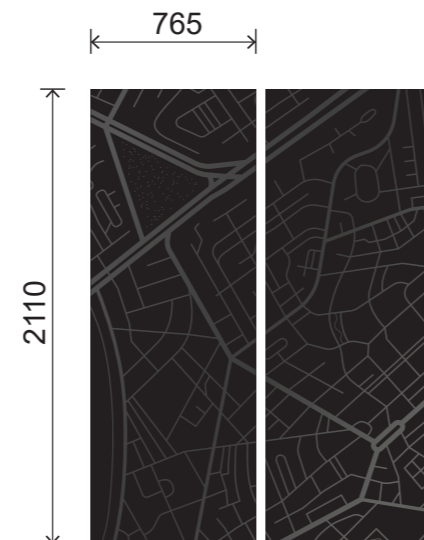
SIGN 3 SIDE ELEVATION GLAZINGS QTY. 1 Digitally printed road map applied externally to glazing. Apply black matt vinyl first, then apply digitally printed graphics. Size: 765mmW x 2110mmH
