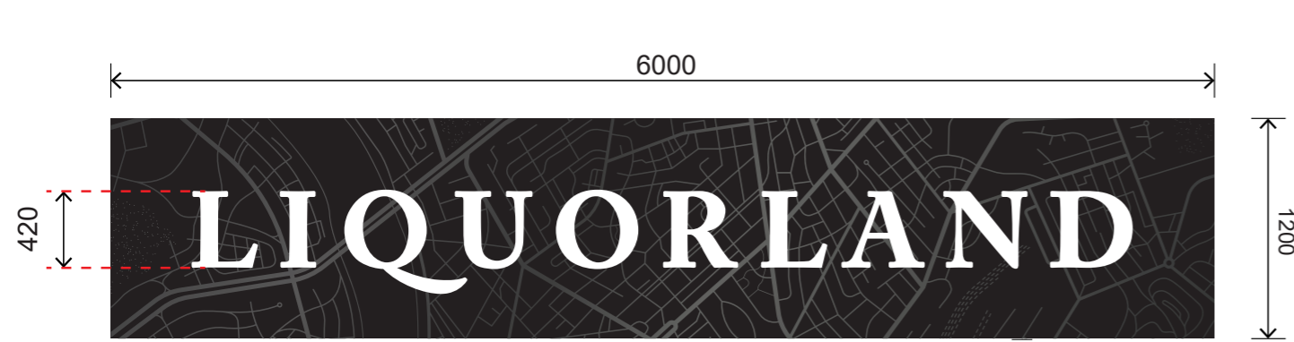
SIGN 1 STORE ENTRY SIGN - Non-illuminated QTY. 1 2mm Aluminium panel with digitally printed black with matt laminate, with all edges to be wrapped. Size: 6000mmW x 1200mmH
