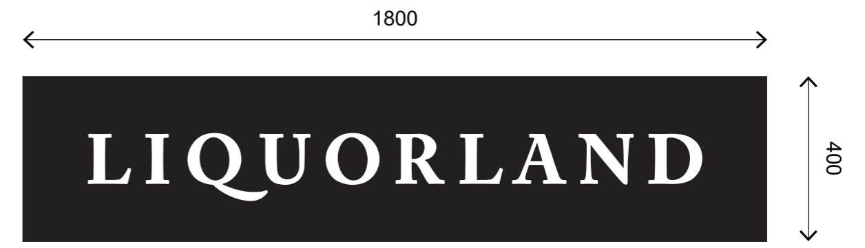
SIGN 6 UNDER AWNING D/S SIGN QTY. 2 4.5mm opal acrylic with black matt CCV. Upgrade LED's. Paint box black. Approx Size: 1800mmW x 400mmH
