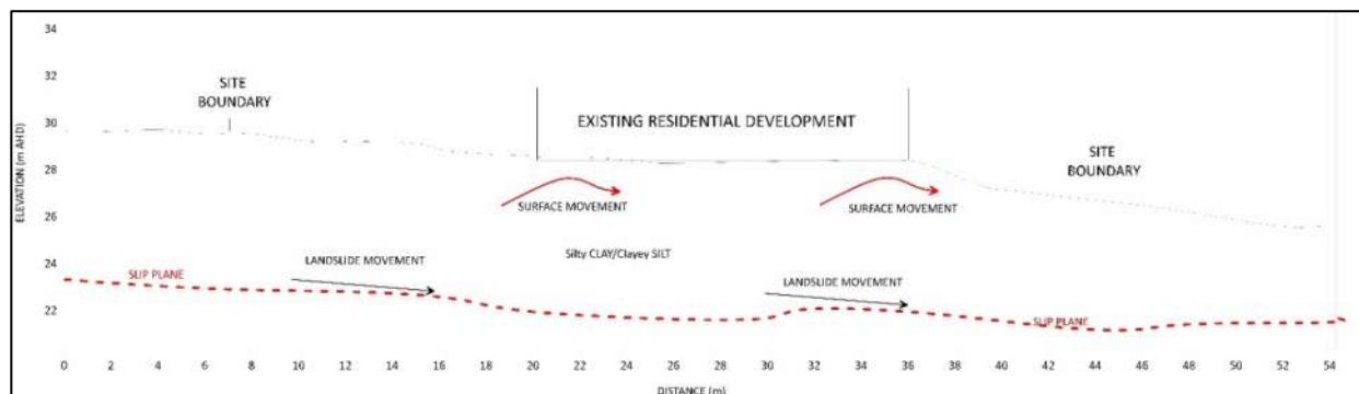
Figure 9 - Conceptual Cross Section of Slope Failure Mechanism relevant to the site (Not to scale)
