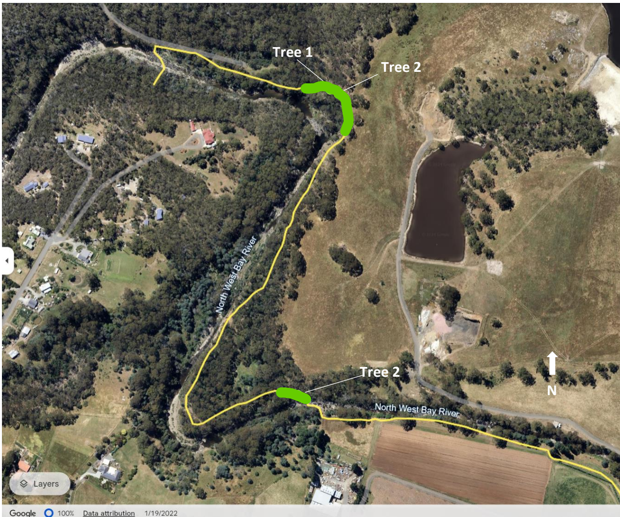
Figure 4. Sections of the North West Bay Track requiring “Medium” or “Heavy Benching” type construction are highlighted in green, as outlined in the North West Bay River Multi-use Trail Feasibility Study. These construction methods have the potential to impact nearby trees.
