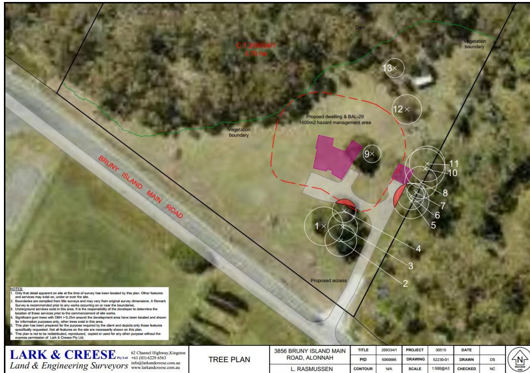
Figure 19 – Image showing proposed location of access and development site extent of proposed 1600m 2 BAL-29 Bushfire hazard management area within land classified as Agricultural / Modified, in proximity to threatened DOV & DTO vegetation communities to the west (see Appendix B for tree register).
