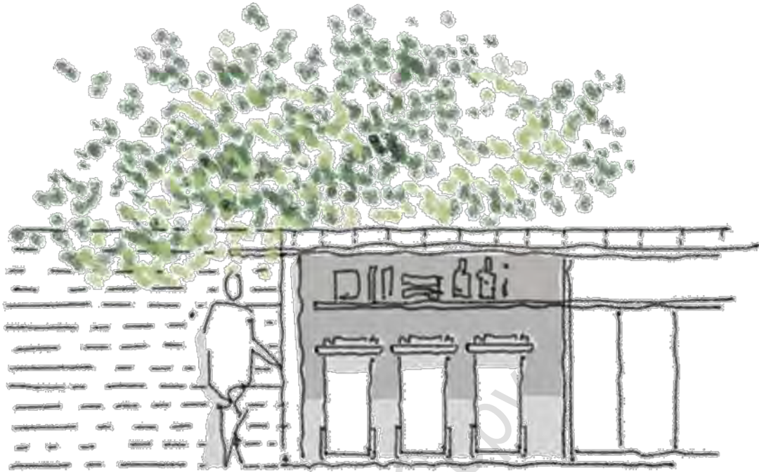
Integrated slimline storage sheds for bin storage and garden equipment.
