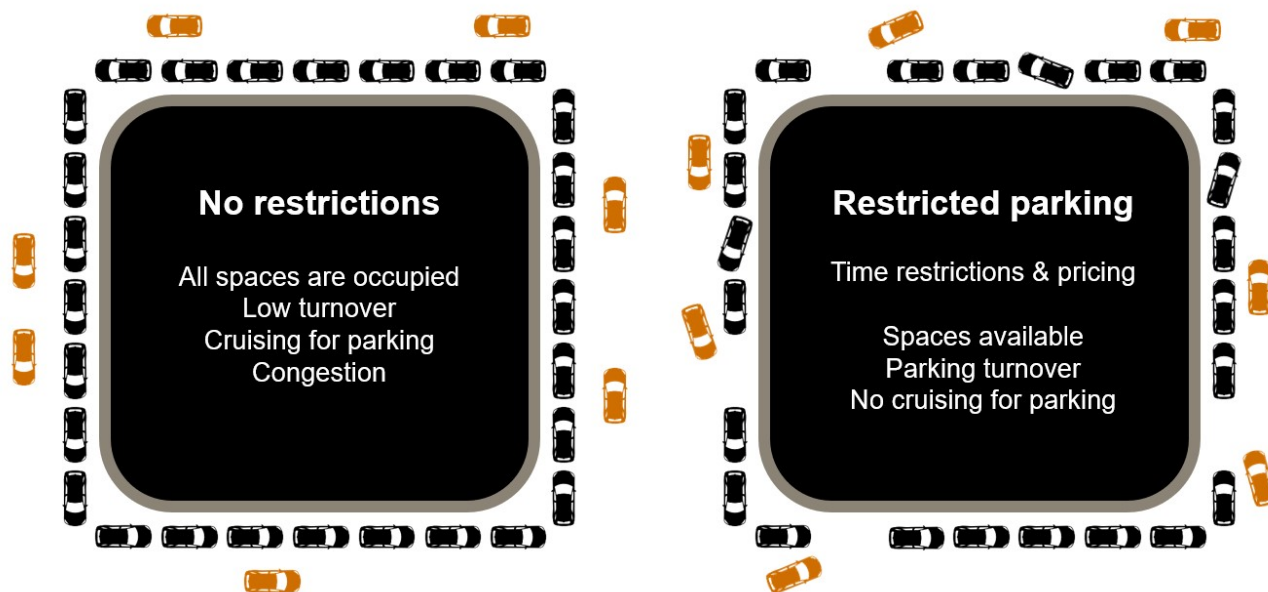
Figure 7.6 – The impact of on-street car parking occupancy on circulation time
